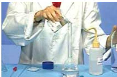
Picture 2 - Transfer the NaOH solution into a 250 mL volumetric flask.
