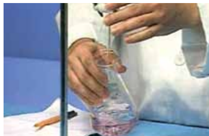
Picture 5 - Titration of KHP with NaOH solution. The pink colour shows that the end point has been reached.
