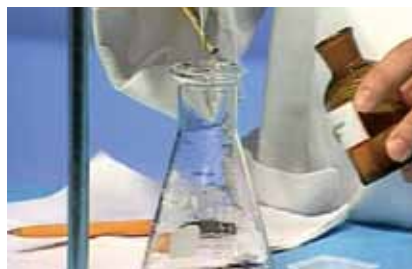
Picture 4 - Addition of phenolphthalein, indicator of the KHP solution.
