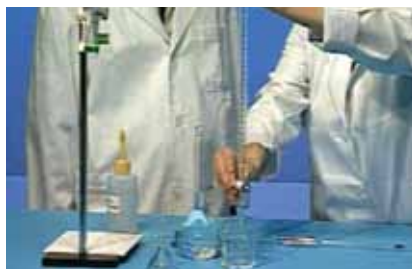
Picture 3 - Rinse and fill the burette with NaOH solution.
