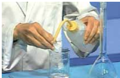
Picture 1 - Dissolve NaOH in deionized water:
