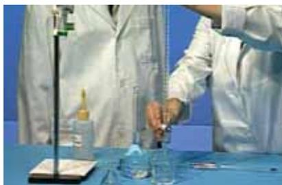
Picture 3 - Rinse and fill the burette with NaOH solution.
