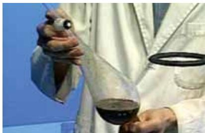
Picture 2 - Extraction of caffeine with dichloromethane in the separation funnel.
