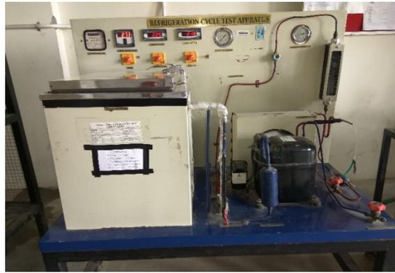
Figure 2: Laboratory setup of the VCRS test rig
