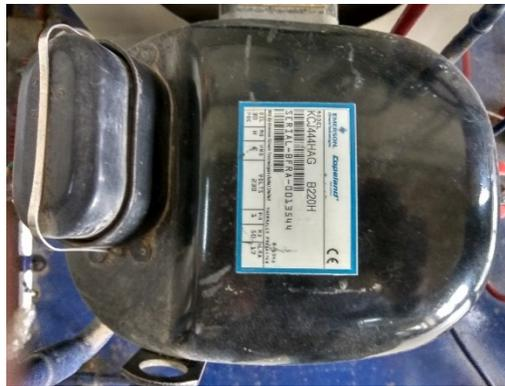
Figure 3: Compressor of the VCRS test rig
